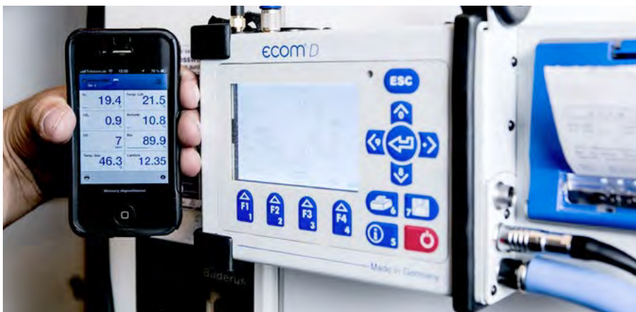
Free hand thanks to Wi-Fi data transfer Data transmission and process on smartphone or Laptop/PC (Apps + software free of charge)
