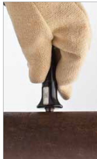
D790-SM Transducer on high-temperature pipe
