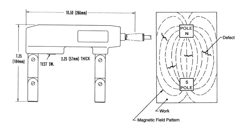
**INSTRUMENT DESCRIPTION:** Basically the B300 Contour Probe is an electromagnet producing a strong AC magnetic field. Placement of the two poles (legs) upon ferrous materials merely provides a path for the intense magnetic field to pass from one pole to the other. The part completes the flux path and becomes highly magnetized.
