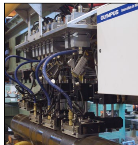
One of the Aqualene's many uses: phased array probe cluster used in an Olympus industrial pipe inspection system.
