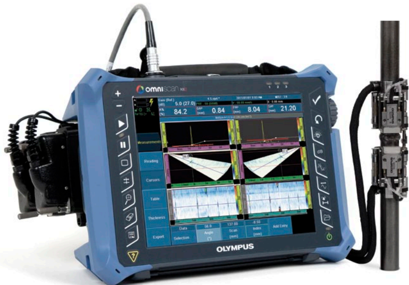
The COBRA scanner on a 0.84 in. pipe with two A15 PA probes with an OmniScan MX2 16:64 displaying two PA groups with sectorial scans, A-scans, and C-scans.
