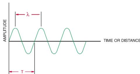
The number of cycles completed in one second is called frequency (f) and is measured in Hertz (Hz), with multiples as follows;
