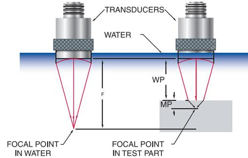
This change in the focal length can be predicted by Equation (13). For example, given a particular focal length and material path, this equation can be used to determine the appropriate water path to compensate for the focusing effect in the test material.
