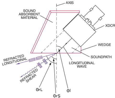
The incident angle necessary to produce a desired refracted wave (i.e. a 45° shear wave in steel) can be calculated from Snell's Law as shown in Equation (12). Because of the effects of beam spread, this equation doesn't hold at low frequency and small active element size. Contact us for details concerning these phenomena.
