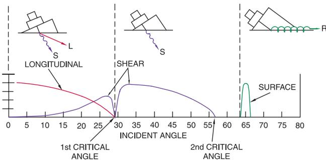
Angle beam transducers are typically used to locate and/or size flaws which are oriented non-parallel to the test surface. Following are some of the common terms and formulas used to determine the location of a flaw.
