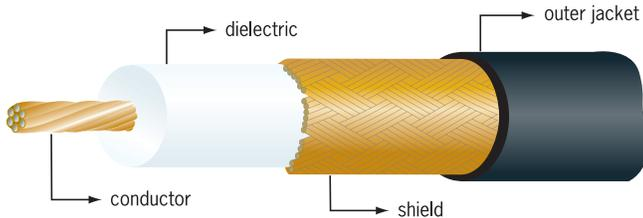
Most cables have one shielding/braided layer. However, to better prevent electrical interference from the environment double shielded cables have an additional shielding/braided layer in contact with the other.
