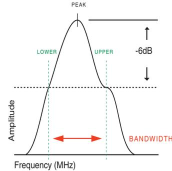
The relation between MHz bandwidth and waveform duration is shown in Figure (6). The scatter is wider at -40 dB because the 1% trailing end of the waveform contains very little energy and so has very little effect on the analysis of bandwidth. Because of the scatter it is most appropriate to specify waveforms in the time domain (microseconds) and spectra in the frequency domain.
