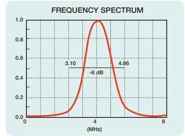
Signal waveform and frequency spectrum of AM4R-8X9-45
