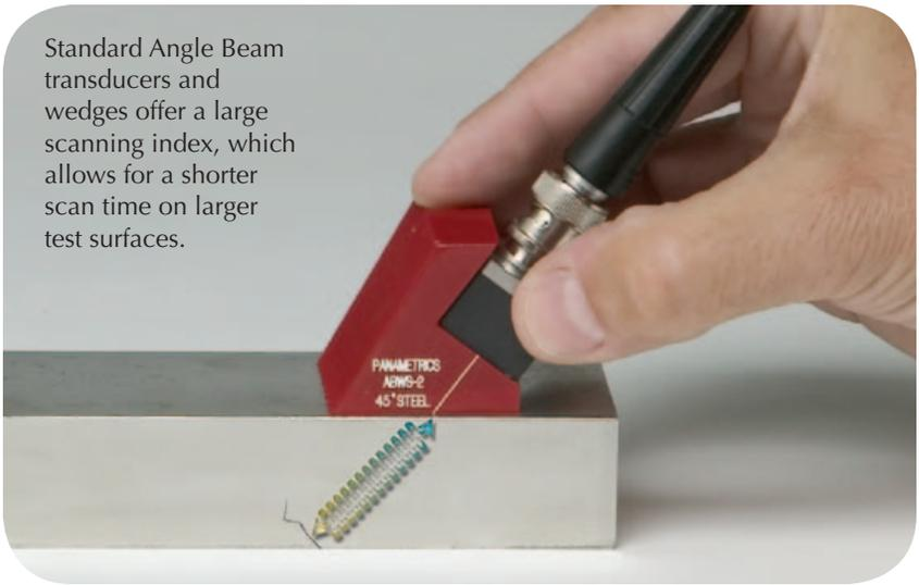
Standard Angle Beam transducers and wedges offer a large scanning index, which allows for a shorter scan time on larger test surfaces.
