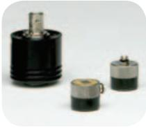
**Contact Transducers:** A contact transducer is a single element transducer, usually generating a longitudinal wave, that is intended for direct contact with a test piece. All contact transducers are equipped with a WC5 wear face that offers superior wear resistance and probe life as well as providing an excellent acoustic impedance match to most metals. Please see page 6 for more details on longitudinal contact probes or page 15 for information on normal incidence shear wave transducers.
