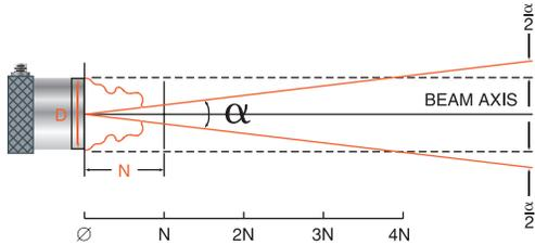
For flat transducers as shown in Figure (10), the - 6 dB pulse-echo beam spread angle is given by Equation (11):
