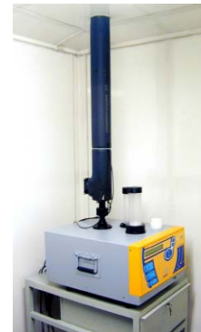
SWAM 5A installed
