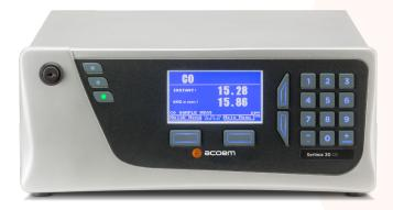
The Serinus<sup>®</sup> 30 carbon monoxide (CO) analyser delivers precise and reliable performance at excellent value. It uses proven NDIR gas filter correlation technology to measure CO in ambient air (LDL < 40 ppb, range 0 to 200 ppm).
