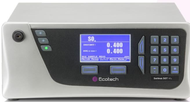
**The Serinus<sup>®</sup> 50T Trace Sulfur Dioxide (SO<sub>2</sub>) analyser delivers precise and reliable performance at excellent value. It uses proven pulsed UV fluorescent radiation technology to measure SO<sub>2</sub> in ambient air (LDL 100 ppt, range 0 - 2000 ppb).**
