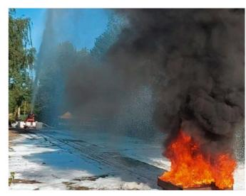
Fire tests for kerosene liquid fires were conducted and documented under the direction and supervision of FlameCert.
