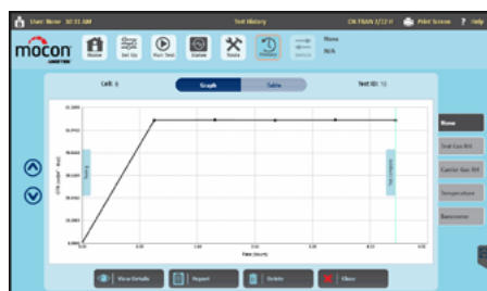
Auto-test mode automatically adjusts the testing parameters to provide results for unknown samples
